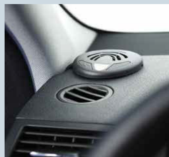
Loudspeaker with LED display (acoustic and visual warning)
