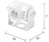
Dimensions Operating voltage Power consumption Image sensor Resolution Picture angle Light sensitivity Video standard Operating temperature Vibration resistance Weight Brightness adjustment Mirrored picture function Protection class Test marks 80 x 75 x 62 mm (incl. mount) 11 to 16 volts DC Approx. 4.8 watts (with heater) 1/3" CCD 290,000 pixels 120° diagonal, h: approx. 108°, v: approx. 92° < 1 lux PAL PAL -30°C to +65°C 10 g 300 g electronic can be set IP 69K E-certificate
