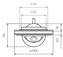
78.5 x 50 mm (incl. installation depth) 12 volts DC approx. 1.2 watts 1/3" CCD sensor 310,000 pixels 125° diagonal; h: ca. 95° v: ca. 70° 0.01 lux -20°C to +50°C 6 g 300 g electronic can be set
