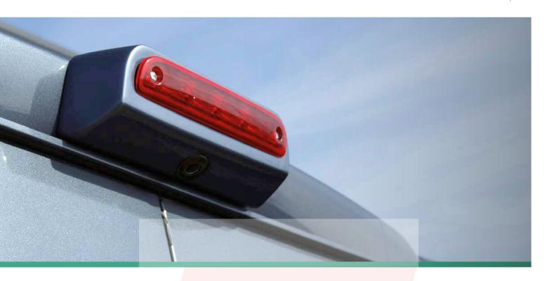
**For Fiat Ducato and its sister models** Citroën Jumper and Peugeot Boxer (from year 2006) we have designed the special camera CAM 29BK. The small cylinder camera is enclosed in a console which is easily installed on the original brake light of the vehicle.
