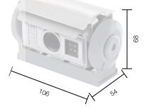
106 x 68 x 54 mm (incl. mount) 11 to 16 volts DC 1.8 watts with heater 1/3" CCD 290.000 pixels 145° diagonal, h: approx. 100°, v: approx. 72° < 0.5 lux, 0 with LED PAI -20°C to +65°C silver 6 g 350 g electronic can be set IP 68 E-certified, ISO 16750
