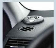
Loudspeaker with LED display (acoustic and visual warning)
