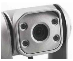
Separately placed LEDs for glare-free night vision
