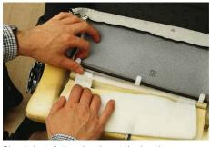
Simple installation: just insert the heating elements between the foam core and the cover
