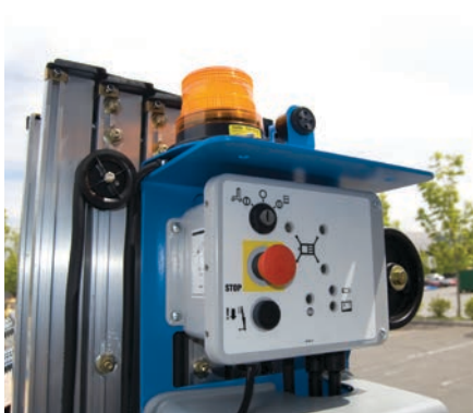
Operational Warning Light
